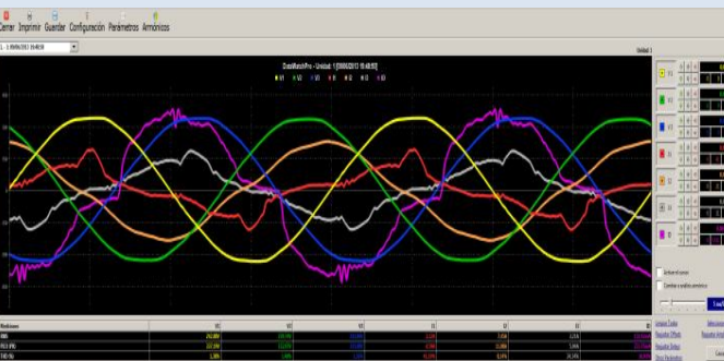
• Module: 6-channel oscilloscope event-logger in waveform with pre-trigger and autoscale (optional).
